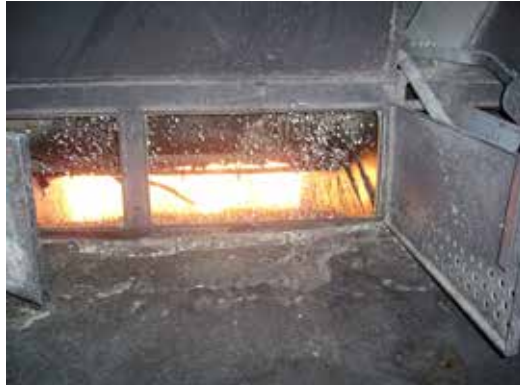
Figure II.9.6: Incineration of sunflower seed hulls at a biodiesel plant (Photo: László Simon)
