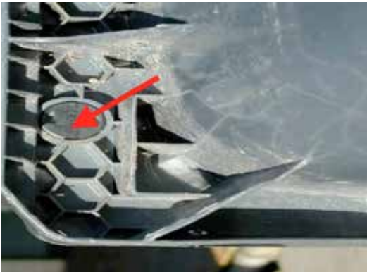
Figure I.4.13: RFID tag fixed under the hinge of the cover of a plastic bin (Rácz, 2010)
