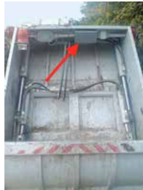
Figure I.4.14: RFID reader device located on the back side feeding mechanism of the waste collection vehicle (Keszthelyi and Vönöczky, 2009)
