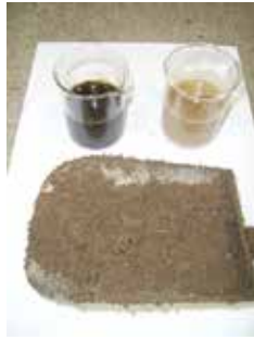
Figure II.10.16: Solid meat sludge (front), fat (left, at the back) and gluey liquid (right, at the back) (Photo: László Simon)
