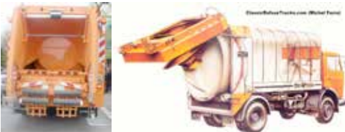
Figure I.4.10: Rotopress type special waste transportation machine (with a revolving drum) ( www.topola.com and www.classicrefusetrucks.com )
