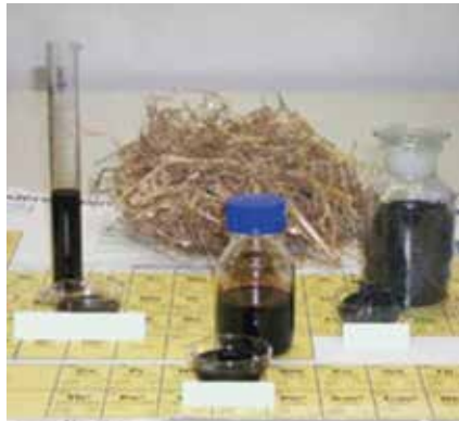
Figure II.9.2: Products created through pyrolysis (in the background: plant parts that have undergone pyrolysis, in the left: pyrolysis oil, in the medium: pyrolysis sludge, in the right: pyrolysis coke)
