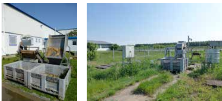
Figure II.11.4: Sieve bend (on the left), and settling, filtering and slack lime feeding unit (on the right) in front of the poplar filtering field (Photo: Zsuzsanna Uri)
