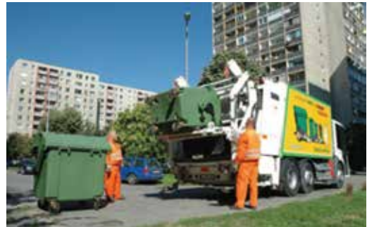
Figure 1.4.3: The collection of municipal waste with a dust-free emptying system ( www.fkf.hu )
