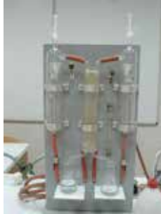
Figure II.13.3: Parnas-Wagner water vapour distillation equipment for ammonia distillation for determination of raw protein content
